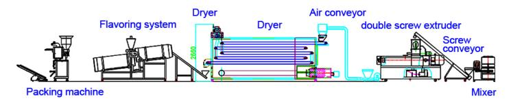
Flow Chart For Automatic Twin Screw Extruder Machine Production Line snack extruder machine corn puff extruder machine
